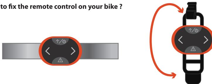
Wrap the silicon strap of remote control around the handlebars of your bicycle.
