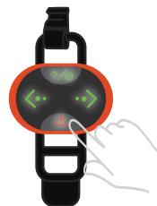
4. The LEDs of the remote and panel will turn on if pairing successful
